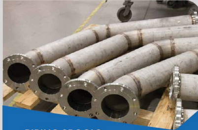
PIPING SPOOLS FABRICATION
